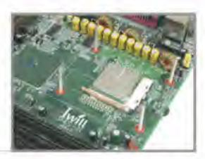
Place and tighten four nuts all the way down.
